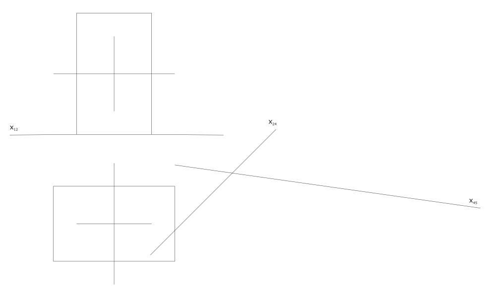
There are three mutually perpendicular golden rectangles given in the figure. Number the vertices  $1 \dots 12$ . Extend the figure to regular icosahedron. Construct two consecutive transformed images with respect to the axes  $x_{24}$  and  $x_{45}$ . show the visibility.
