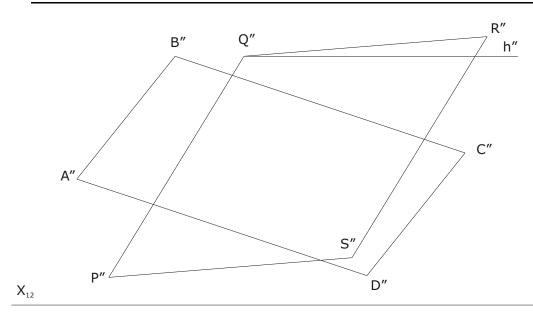
Construct the line of intersection of the two given plane figures using the method of auxiliary projection for special purposes.
