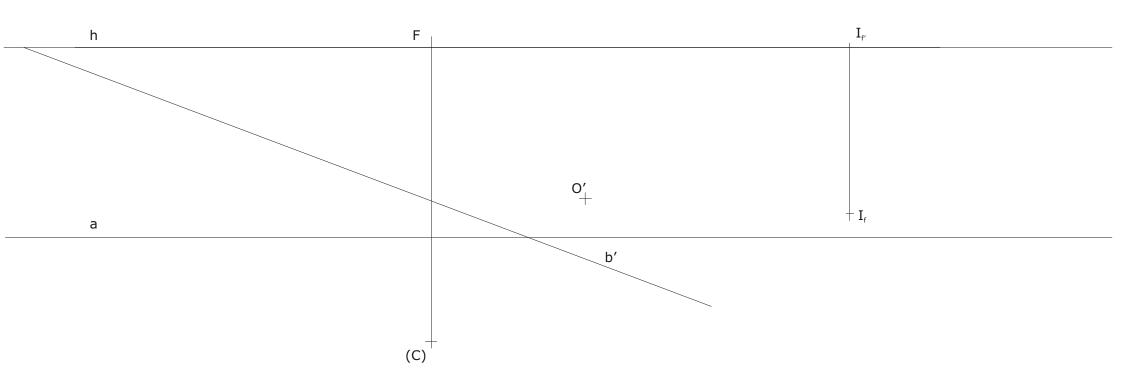
Represent a prism with regular hexagon base in perspective with vertical picture plane. The center of the hexagon is the point O, one of the sides lies on line b, and the height of the prism is 82 mm. Remove the lateral face, closest to the observer (centre of perspective). Show the visibility of the surface that consists of the base hexagon, lateral faces and the top face. Construct all shadows and shades at parallel lighting given by  $I_f$  and  $I_f$ .
