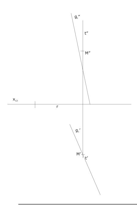
Construct the intersection of a right circular cone with vertical axis and a plane given by its gradient line  $g_1$ . The radius of the base circle is r, the vertex of the cone is M.
