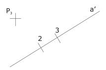
4. Construct parallel line to the given line a trough the point  $P_{\scriptscriptstyle 5}\,.$
