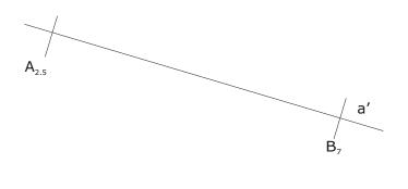
3. Construct the level lines of the given plane (axb).
